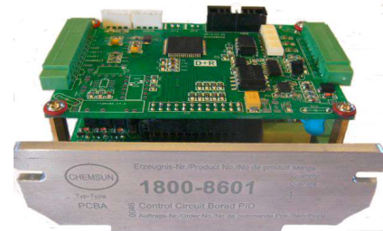
Fig. 11: Actuator master control board and interface board
